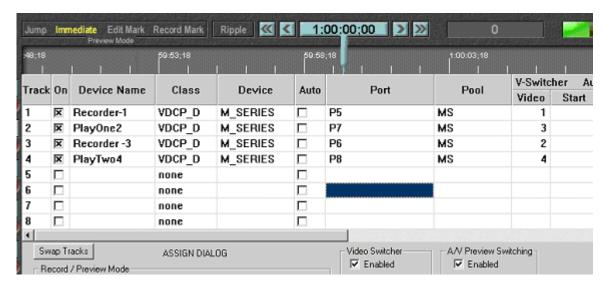
In the example above, the Device Name assigned to Track 1 is **Recorder-1**. The ( - ) minus defines this channel as a Recorder channel, and the "1" defines this channel as Protocol Control Port 1. The name "Recorder" can be replaced by any descriptive name that does not contain a ( - ) minus or the numbers 1 through 4.
